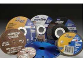
The Norton small diameter cut-off wheel line consists of Type 01/41 straight and Type 27/42 depressed center cut-off wheels from 1-1/2" to 9" diameters. These wheels come in ultra thin .035 for quick burn-free and burr-free cutting to .125" for more durable applications. All are reinforced for the demanding nature of portable cut-off.
